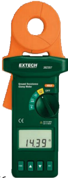
Verify resistance of cellular and communication tower ground grids
