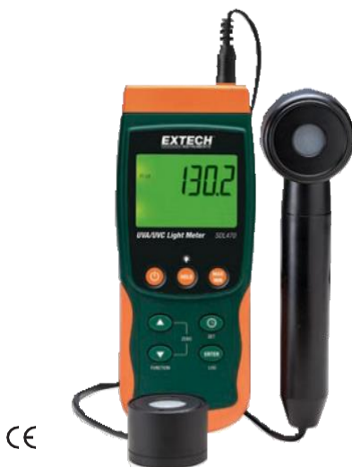
Complete with built-in tilt stand, SD memory card, UVA light sensor with protective cover, UVC light sensor, hard case, Universal AC adaptor, and 6 x AA batteries
