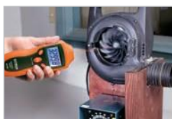
Measures the speed (RPM) of rotating objects and counts (revolution) of moving objects.
